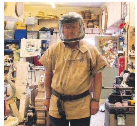
▲ Pic.9 Protection is always important when working with wood but the dust from plywood can be particularly unpleasant, so smock, work boots and a full respirator is desirable
